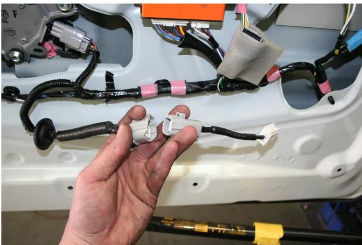
4. Remove jack from storage area, and make a small cut in either end of original rubber conduit. Feed camera loom through as per photo.
