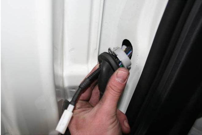
5. Remove rubber grommet from under left side of vehicle.
